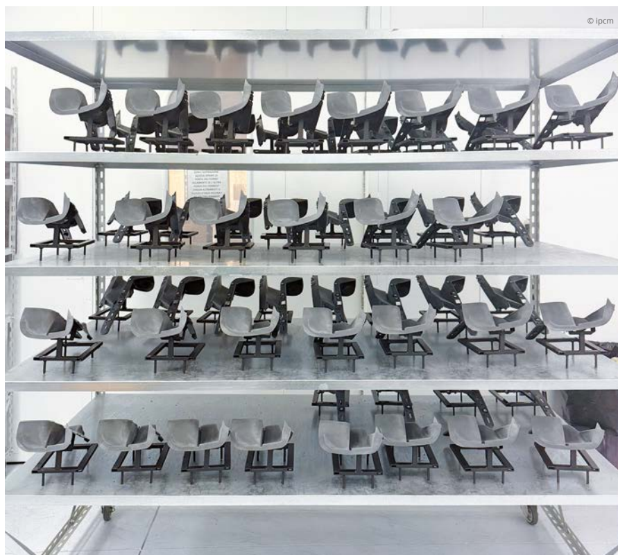
Components arranged on the special racks designed by Quality Painting.
