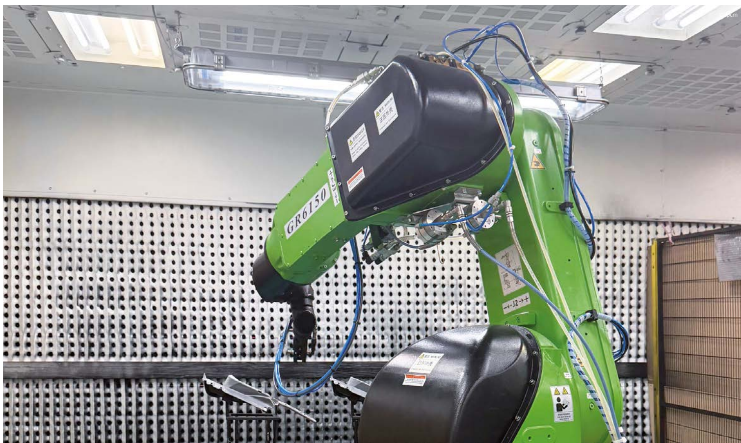
The automatic mixing system integrated directly onto the robot arm, with gear pumps and valves for colour change, which conveys the paint products from the management units to the application point.
