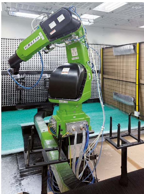
The self-learning coating robot supplied by CMA Robotics.
