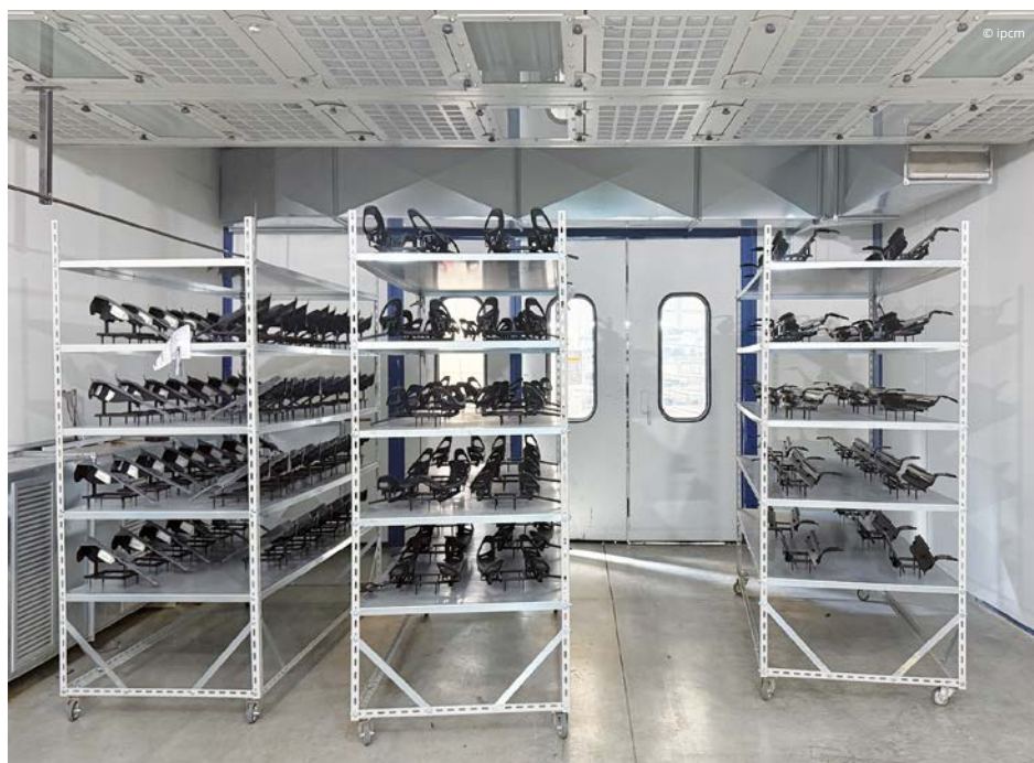
After application, the components are taken to the baking oven, where they dwell for at least 1 hour at a controlled temperature.
