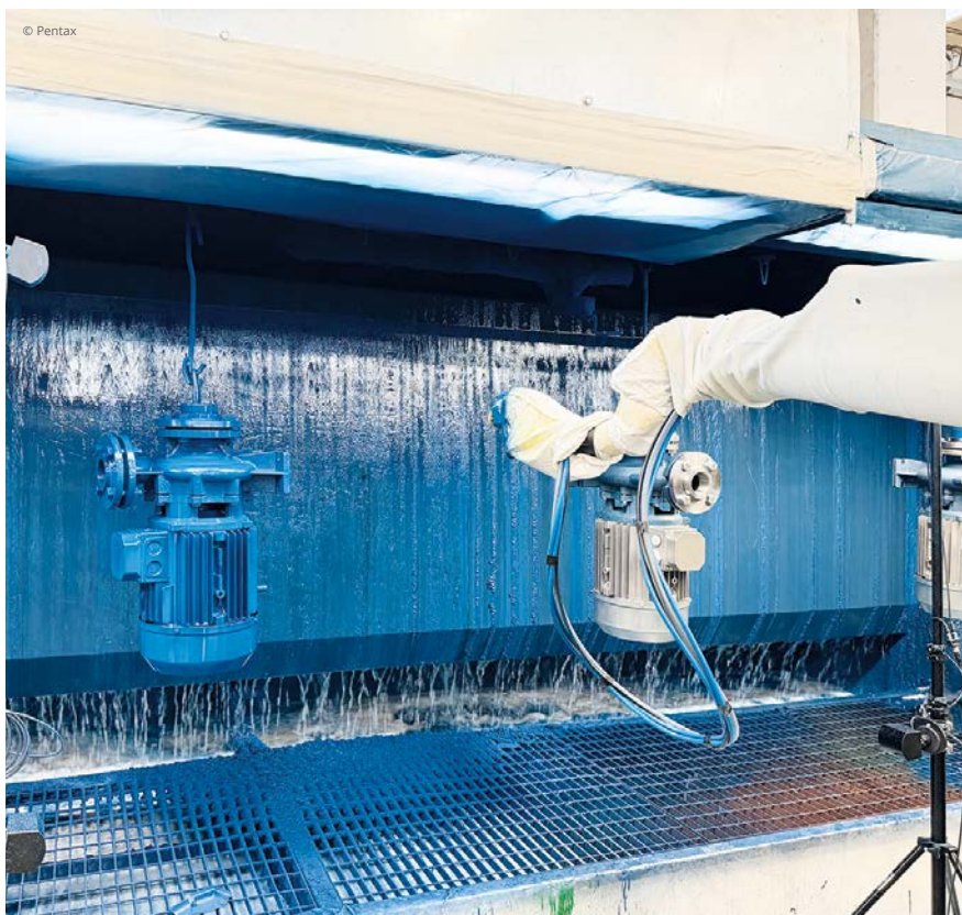
Coating application via an articulated robot.
