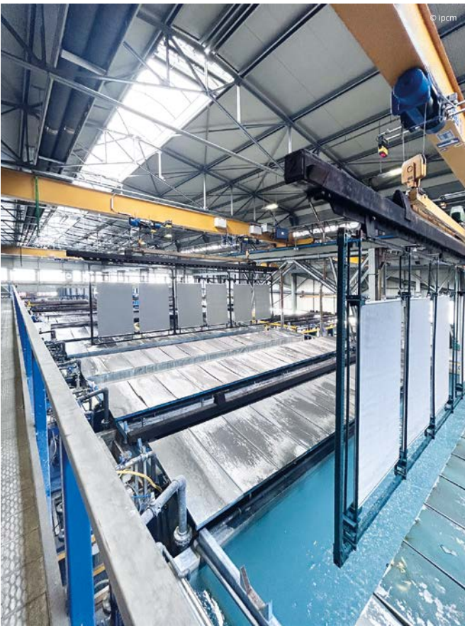
The cataphoretic coating is applied by dipping at Modine's San Vito al Tagliamento plant in Italy.
