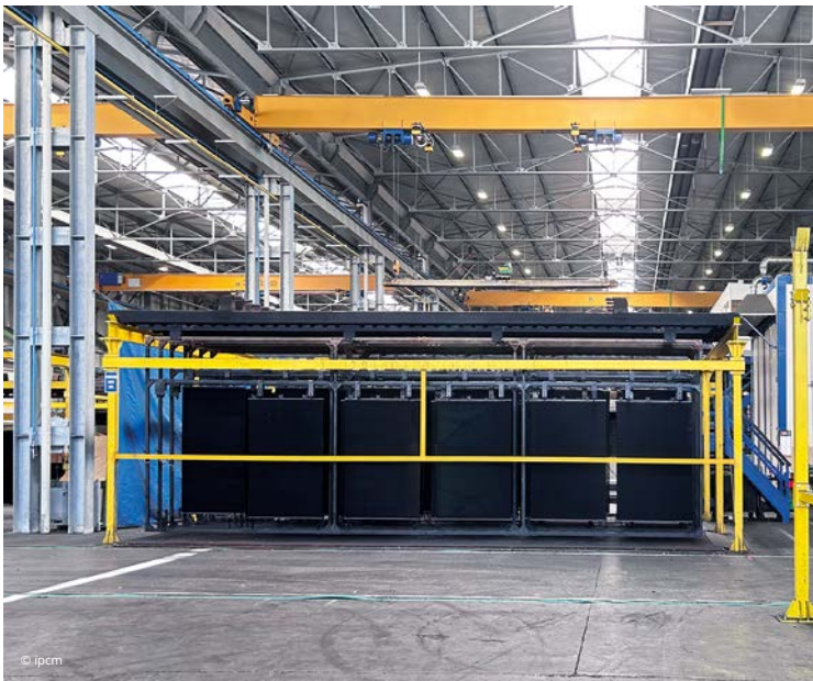
The storage buffer for parts awaiting unloading before packaging and final dispatch.
