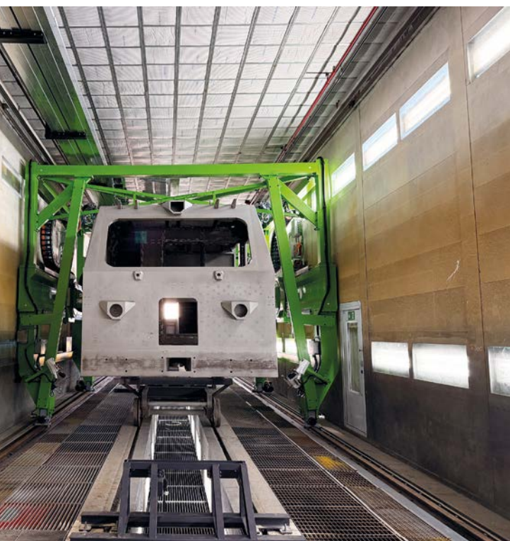
In the coating booth, MERMEC Ferrosud uses robots to apply an anti-rust primer, a sandable acrylic primer, and a polyurethane top coat. On the left, the metal gantry equipped with two 9-axis GR-6150 articulated robots from CMA Robotics.
